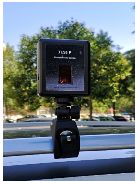
Illustration 7: With the appropriate accessory it is possible to attach the sensor to the car to take measurements on the road.
