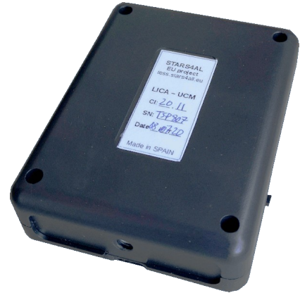
Illustration 4: Calibration label. Each photometer is calibrated at LICA UCM laboratory.
