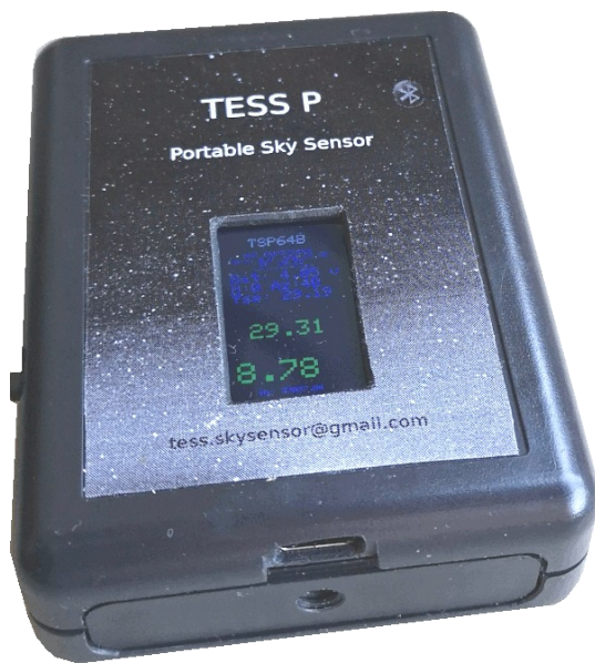
Illustration 1: TESS-P front with color display. At the bottom USB C connector and 1/4 thread for tripod.
