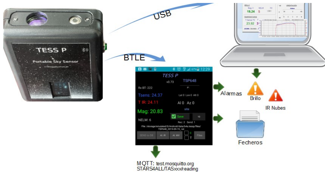
Illustration 5: TESS-P communication options: BT and USB. With USB it is possible to record the brightness evolution of a whole night. In both cases it is possible to activate alarms.
